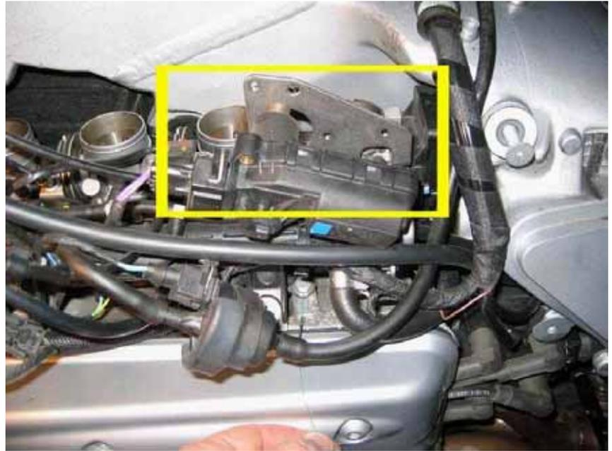
The last spring is accessed from below. You need to hook the loop from below, then relax the end upward on the inside to its new position.
