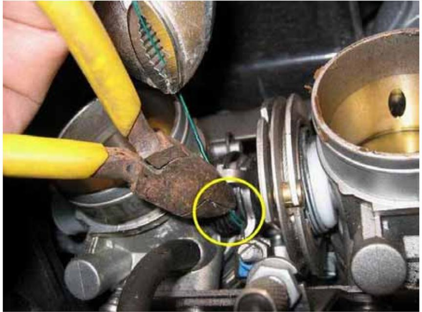
**After the loop is snipped, gently remove it from under the spring. Take care to not pull the end of the spring off the mount. It looks like it would be a real pain to recover from that screw-up.**
