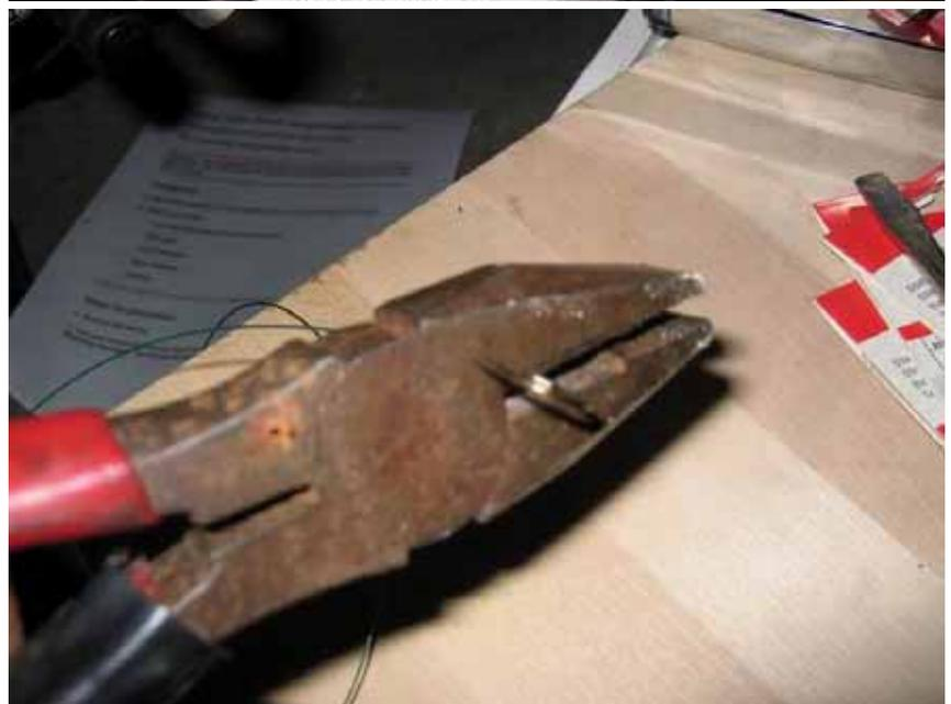
Use a small vice grip pliers to hold the loop end of the leader. As you can see here, you only need an inch or two protruding from the end of the pliers.
