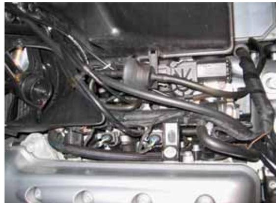
After you remove the gas tank, loosen the air duct (on the right side of the bike) which inserts into the upper right part of the airbox. The airbox is attached underneath to the four (4) throttle bodies with four clamps. Loosen these clamps and then pull the airbox straight up.
