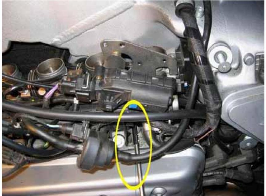
**This bottom picture is a bit hard to see, so I stretched it out a bit. You should be able to see the green leader coming up from below. It is hooked onto the end of the spring. I found it helpful to use a long, thin screwdriver to direct the end around to its final resting place.**
